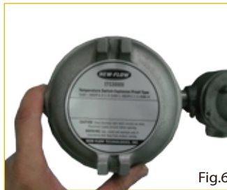
Fig.2: 首先用十字螺絲起子拆開表蓋。 First, open the cover with a cross-head screwdriver.
