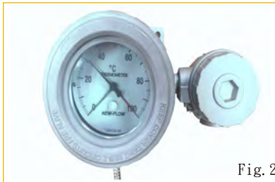
Fig. 2 首先用十字螺絲起子拆開表蓋。 First, open the cover with a cross-head screwdriver.
