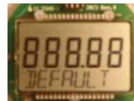
Depress “B”, LCD display “DEFAULT” on lower line and “888.88”on upper line.
