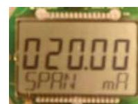
Depress either one of button “A” or/and “B” with referring to the adjusting procedure of “Zero setting (ZERO mA)” until getting the represented number of full span.
