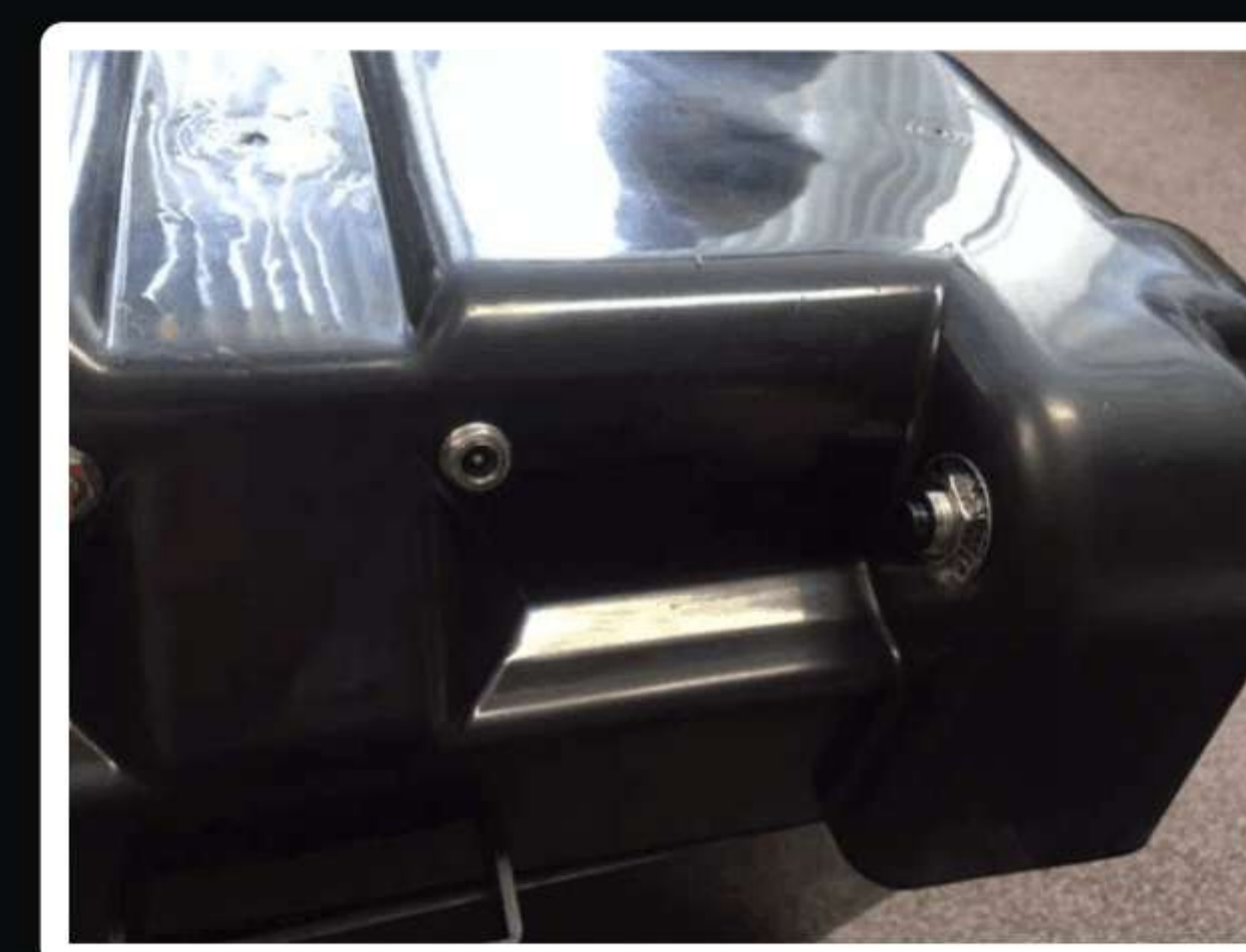
• A 2.5mm DC power jack must be fitted. A Plastic Jack is preferred. • A 10A automotive style circuit breaker must be fitted
