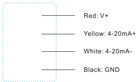
Four wire analog output
