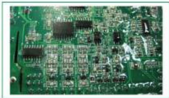
Thick PCBA coating for hard environment using
