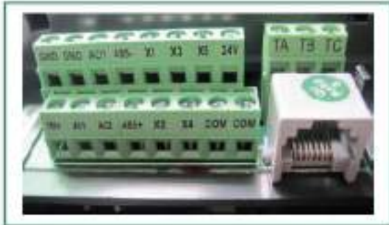
Clear silk print of terminal mark easy for wiring
