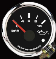
MMOPW-90B(010) ELECTRICAL OIL PRESSURE GAUGE WARNING<0.8BAR W/SENSOR 10~180 OHM / 0-10 BAR
