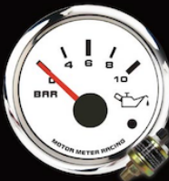
MMOPW-90W(010) ELECTRICAL OIL PRESSURE GAUGE WARNING<0.8BAR W/SENSOR 10~180 OHM / 0-10 BAR
