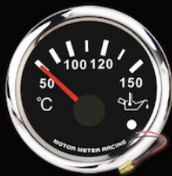
MMOTW-90B ELECTRICAL OIL TEMP GAUGE WARNING>108°C W/SENSOR 362~20 OHM / 50~150°C
