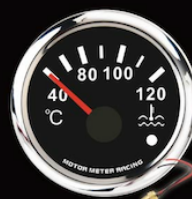
MMWTW-90B(40120) ELECTRICAL WATER TEMP GAUGE WARNING>95°C W/SENSOR 301~22 OHM / 40-120°C
