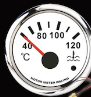
MMWTW-90W(40120) ELECTRICAL WATER TEMP GAUGE WARNING>95°C W/SENSOR 301~22 OHM / 40-120°C
