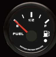
MMFLW-90B-B(0190) MMFLW-90B-B(24033) ELECTRICAL FUEL LEVEL GAUGE WARNING<13% 0-190 OHM 240-33 OHM
