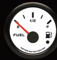
MMFLW-90W-B(0190) MMFLW-90W-B(24033) ELECTRICAL FUEL LEVEL GAUGE WARNING<13% 0-190 OHM 240-33 OHM
