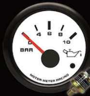
MMOPW-90W-B(010) ELECTRICAL OIL PRESSURE GAUGE WARNING<0.8BAR W/SENSOR 10~180 OHM / 0-10 BAR
