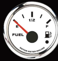
MMFLW-90W(0190) MMFLW-90W(24033) ELECTRICAL FUEL LEVEL GAUGE WARNING<13% 0-190 OHM 240-33 OHM
