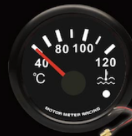
MMWTW-90B-B(40120) ELECTRICAL WATER TEMP GAUGE WARNING>95°C W/SENSOR 301~22 OHM / 40-120°C
