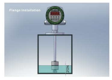
Suitable for tanks with no removable cover. A hole shall be made on the cover according to size of flange. Flange dimension customizable.
