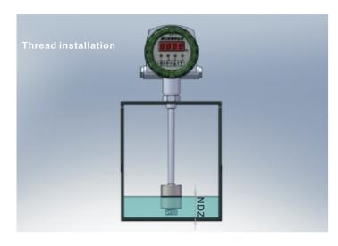
Suitable for tanks with removable cover. Need M20\*1.5 on the cover.
