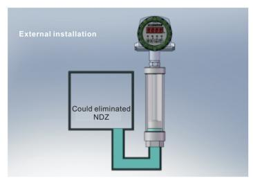
In case that there is no space for installation, an elbow is needed. Elbow and transmitter is connected by G3/4 internal thread.
