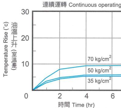
Continuous operated cylinder (Ø20xØ40x250mm)
