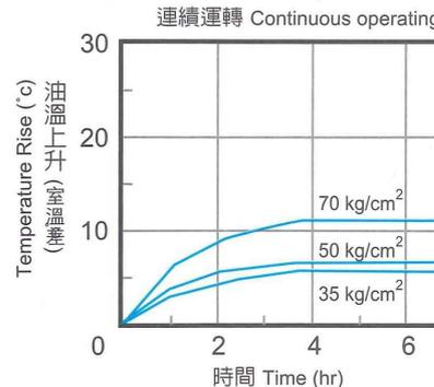
Continuous operated cylinder (Ø20xØ40x250mm)
